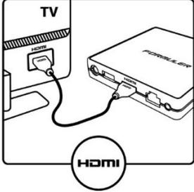
2) Illustration showing the HDMI cable being plugged into the HDMI port of a TV and the HDMI port of a set-top box. The text "HDMI" is in a circle below.
