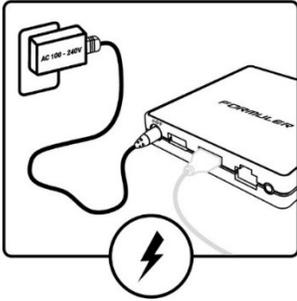
3) Illustration showing the power cord of the set-top box being plugged into a power outlet. A lightning bolt icon is in a circle below.
